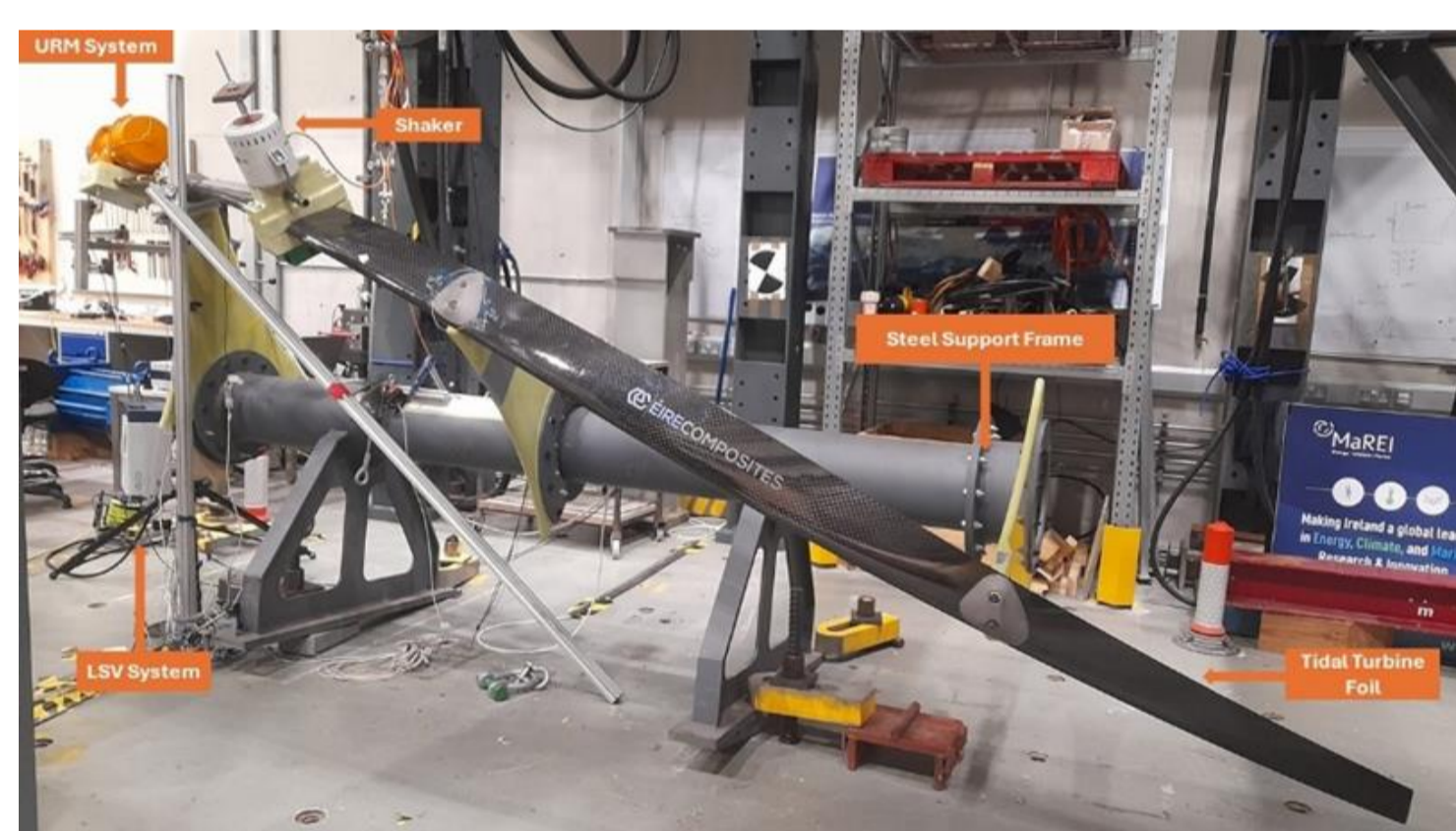
Above: ORPC turbine foil undergoing structural fatigue testing using an unbalanced rotating mass (URM) system at the University of Galway. Image courtesy of the University of Galway
