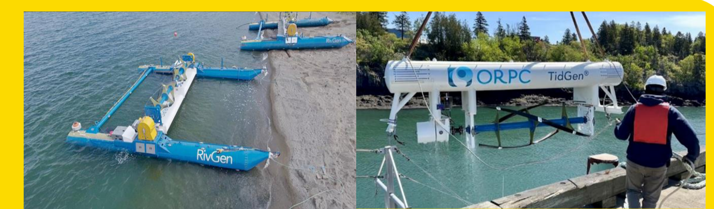
ORPC RivGen® (left) and TidGen® (right) Power Systems
