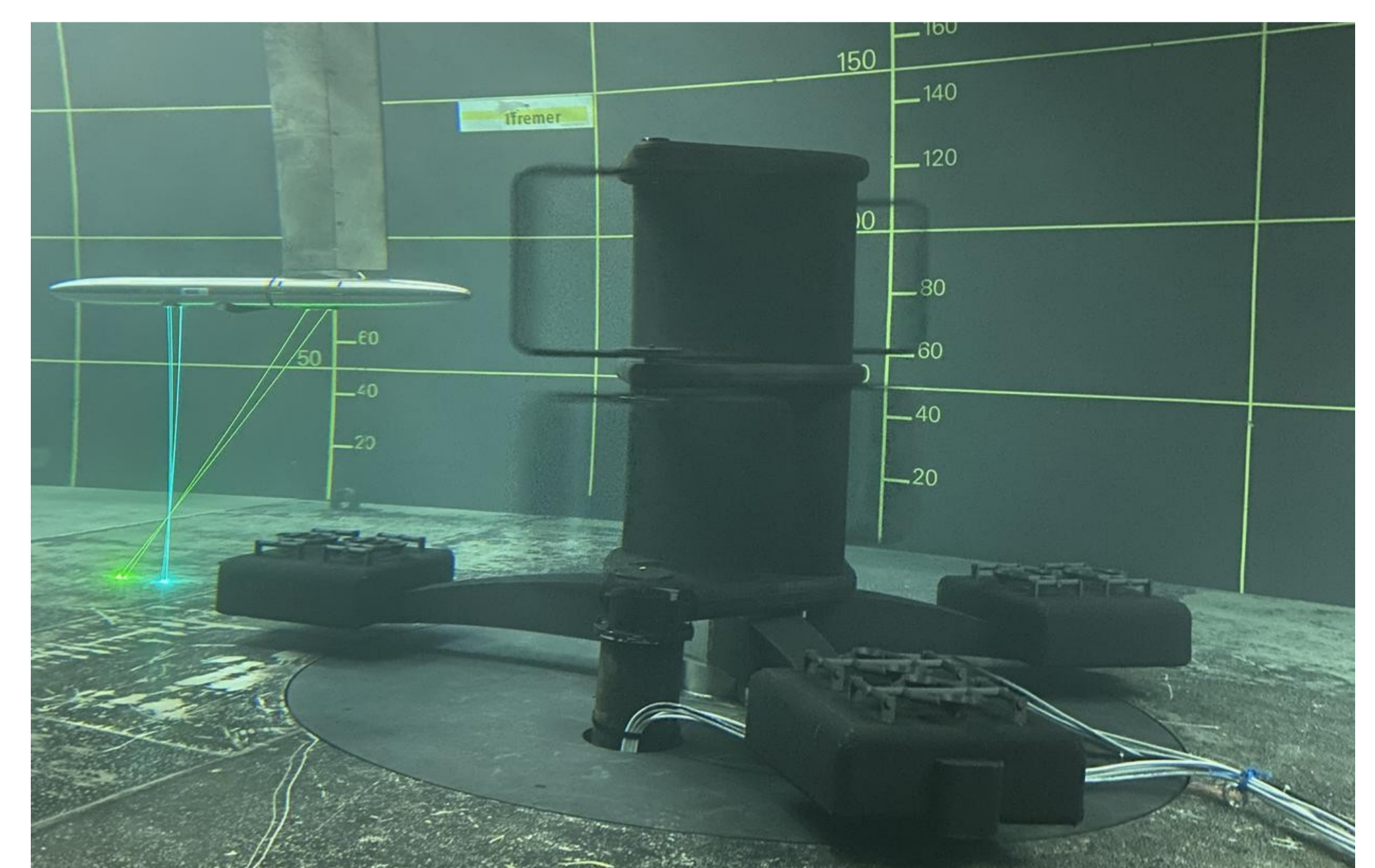
1/20 scale model of the HQ 2.5 in the wave and current flume tank for performance and flow characterization
