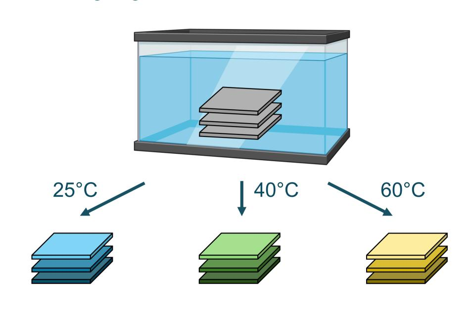
They are then tested to evaluate the change in mechanical properties induced by seawater ageing.
